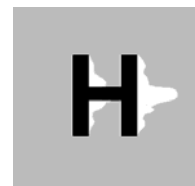
LF too high
