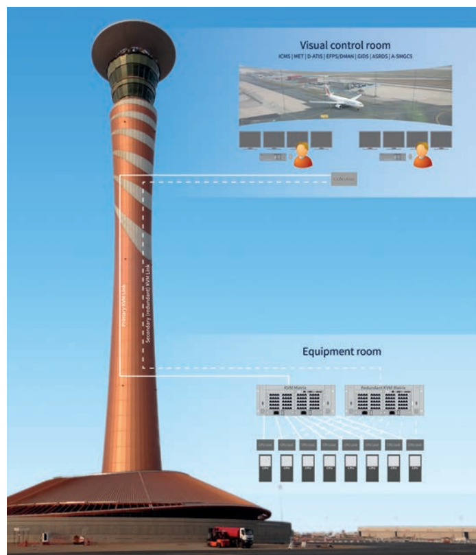
Fully redundant KVM matrix system inside the ATC tower
